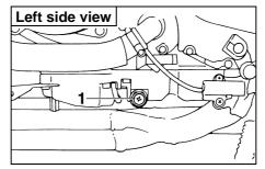
1. Engine oil drain bolt
