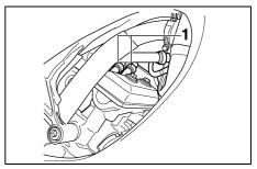
1. Spark plug cap (x 2 on each side)
