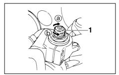
1. Spring preload adjusting bolt
