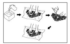
Apply recommended oil to the entire surface of the filter and squeeze out the excess oil. The air filter should be wet but not dripping.
