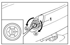
1. Compression damping force adjusting screw
