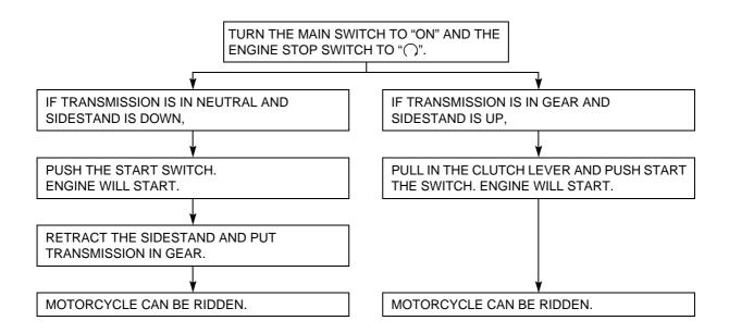
1. Turn the main switch to "ON" and the engine stop switch to "O".
