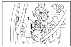
1. Compression damping force adjusting screw
