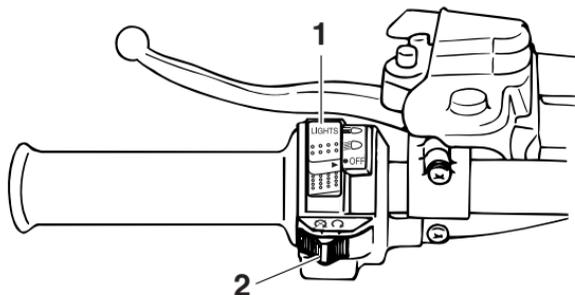
1. Interruptor de luces “ $\text{D}$  /  $\text{L}$  / OFF”
